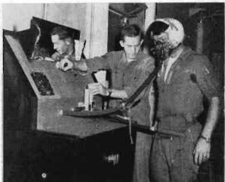
Airman first class Max Pulliam (left), of the 531st, demonstrates the operation of the personal equipment tester that he designed to 1st Lt Niel Udell, one of the 531st pilots. This testing system will test G-Suits up to eight G's on both high and low pressure, test the pilot's headset and mike, and the pilot's breathing apparatus to insure proper performance under pressurized breathing. The tester has a vertical mirror for fitting equipment and a storage cabinet for equipment repair.
